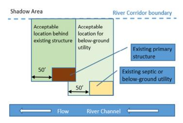
also be placed within the same shadow dimensions of an existing below-ground system.
